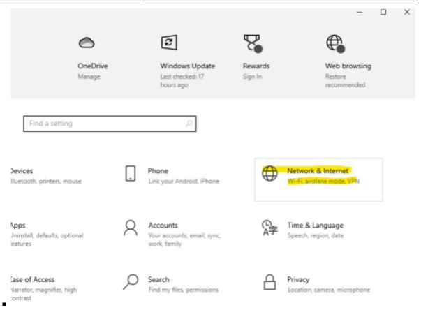
If connected via Ethernet, select Ethernet → Properties. If connected via WIFI select
